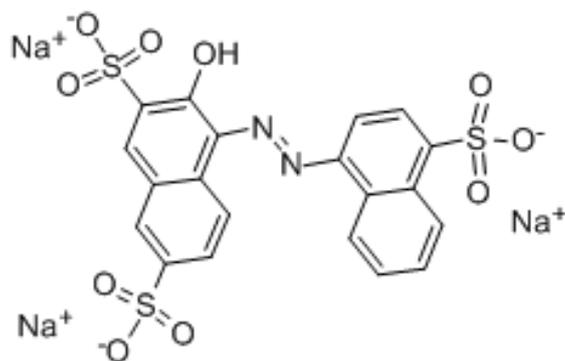
Figure 2.5 Structure du colorant C.I. Acid red 27
