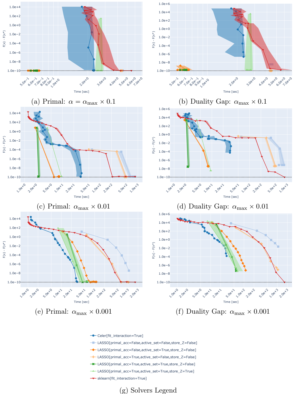
Figure 3.3: Primal convergence on the left and duality gap convergence on the right, with the first sixty columns of Genomics dataset, leading to q = 1830 interactions, for n = 16294 samples. LASSO with Interactions with active set and acceleration are the fastest for the two largest penalties while CELER achieves slightly better in last penalty.
