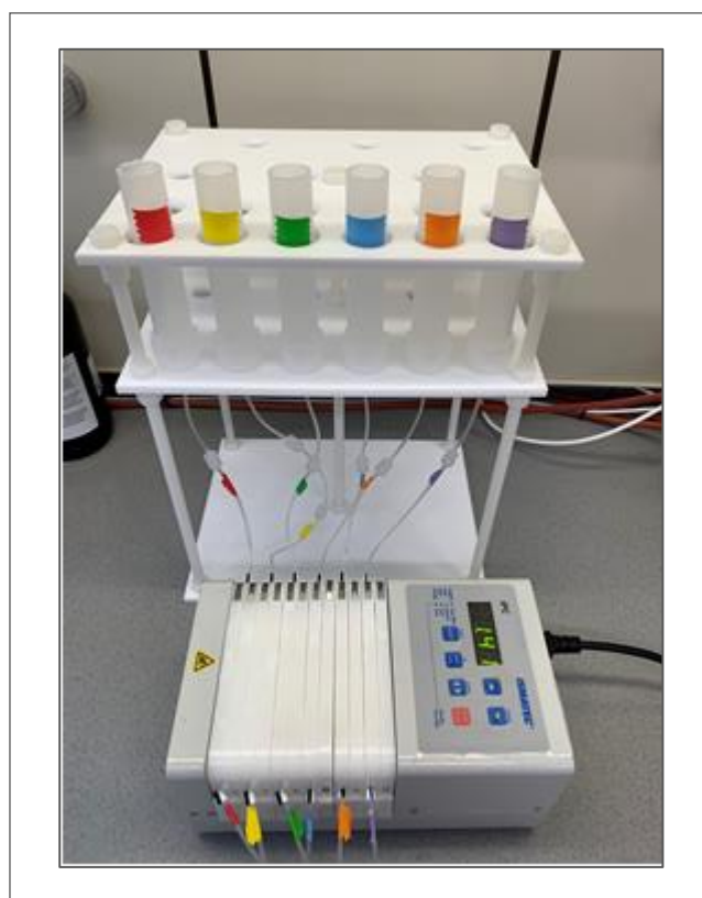
Figure IV.VIII-2: AMP-Cs precipitate filtration system of 6 samples in parallel
