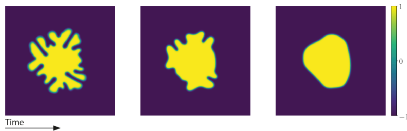
Figure 4.36: Simulation of model C with the coupling parameter \lambda = 0 . The initial condition (on the left) corresponds to a typical shape obtained with \lambda > 0 . The interface smooths out according to motion by curvature dynamics. The other parameters are: dx = 0.6 , dt = 0.01 , L = 250 .
