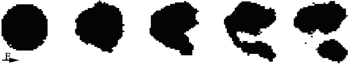
(c) Kinetic Monte Carlo simulation showing the emergence of the splitting instability, for islands that are above a critical size. Image from Ref. [24].
