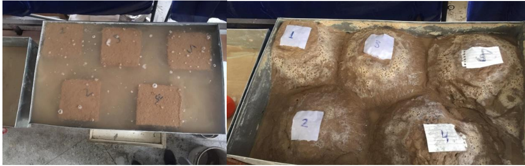
Figure 79: Water absorption and mass loss test on Deh-Sabz CEB, adapted from Varum et al. (2007)
