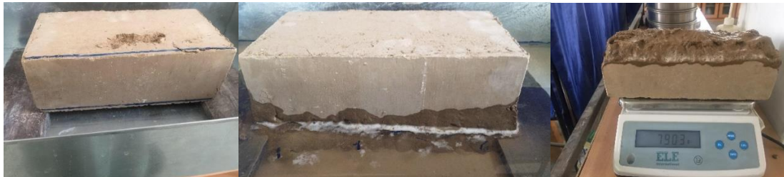
Figure 83: Water absorption and mass loss test (10 and 60 minutes) face down in water on Deh-Sabz CEB
