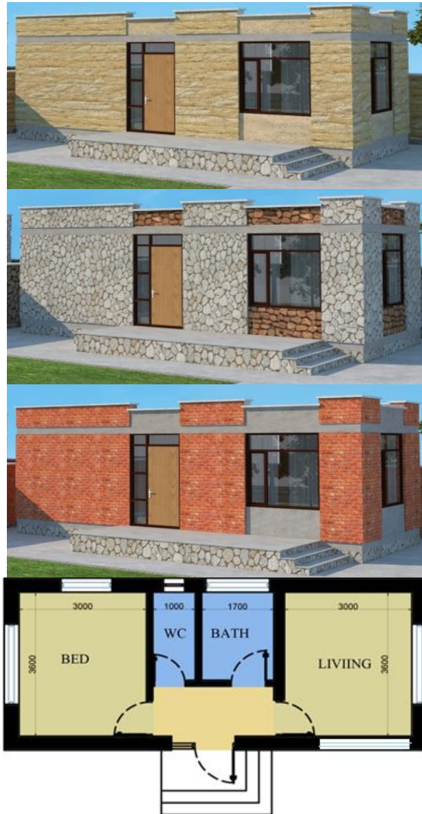
Figure 118: From top: models of incremental housing, using pakhsa, stone, and fired brick (MUDL, 2018)
