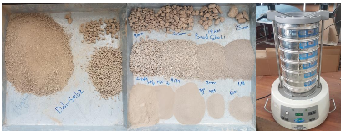
Figure 62: From left to right: dry sieve analysis from Deh-Sabz and Band-e-Ghazi and an automatic shaker (photographs by the author)
