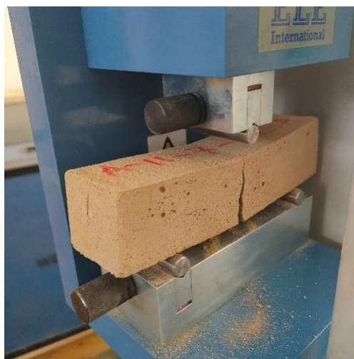
Figure 88: Mix designs A & B flexural strength at 28 days of drying
