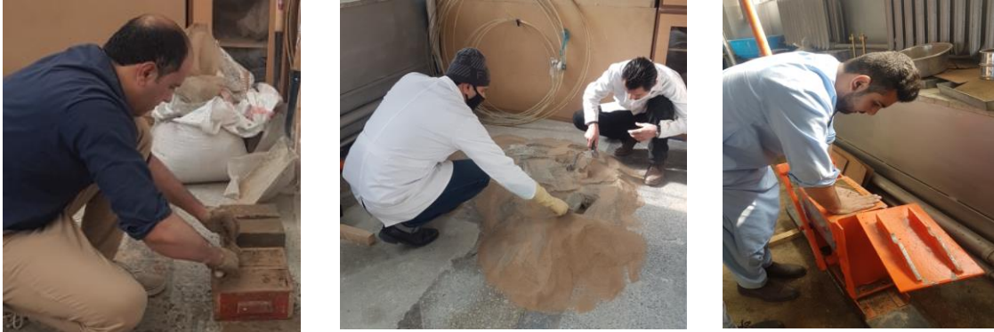
Figure 71: From left to centre/right: production of the sun-dried brick and CSEB
