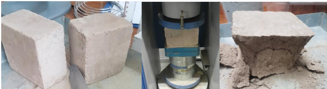
Figure 76: From left to right: saw cutting CEB and compressive strength test
