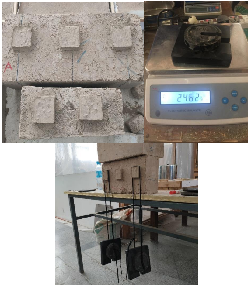
Figure 90: Mortar cohesion test procedure
