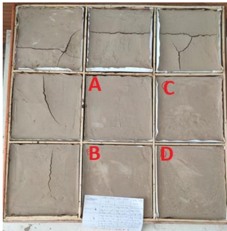
Figure 87: Grid of nine mixtures after a 28-day drying period
