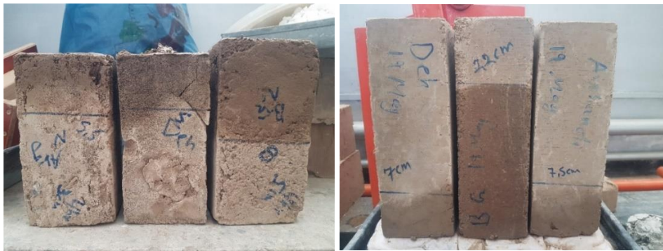
Figure 81: Visual inspection of sun-dried brick and CEB surfaces, after 24 hours on unsaturated cotton
