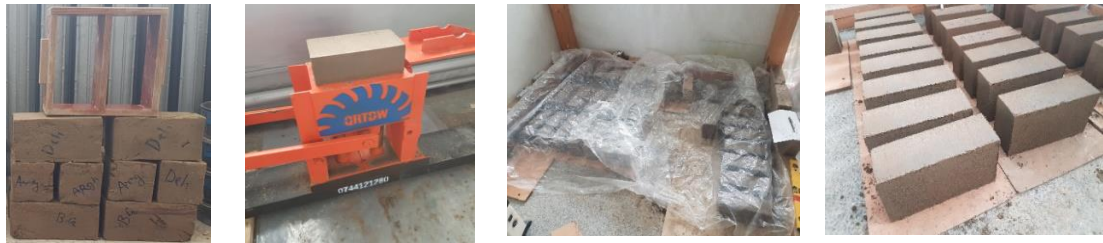
Figure 72: From left to right: initial and final curing of the sun-dried brick, CEB, and CSEB
