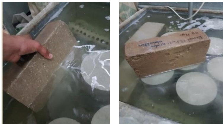
Figure 80: CSEB after 24 hours fully immersed in water
