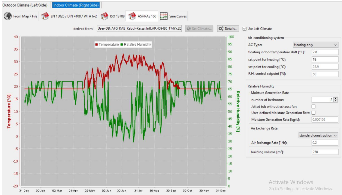
Figure 97: Indoor temperature and relative humidity simulation result for a 500-mm CEB wall, input data from WUFI Pro
