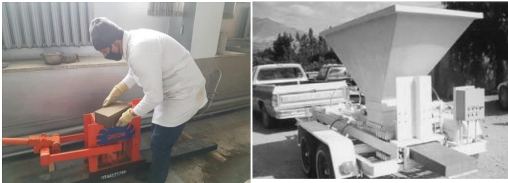
Figure 44: From left to right: manual press block machine (photograph by the author) and automatic block press CLU 3000 (Minke, 2006)
