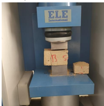
Figure 89: Mix designs A & B compressive strength at 28 days of drying
