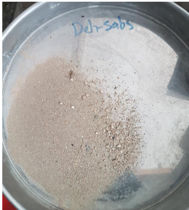
Figure 63: From top to bottom: wet sieve analysis result and remaining sand and gravel after washing Deh-Sabz soil
