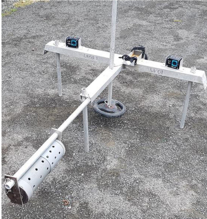
Figure S3: a standard Stereo Baited Remote Underwater Video Station (BRUVS).
