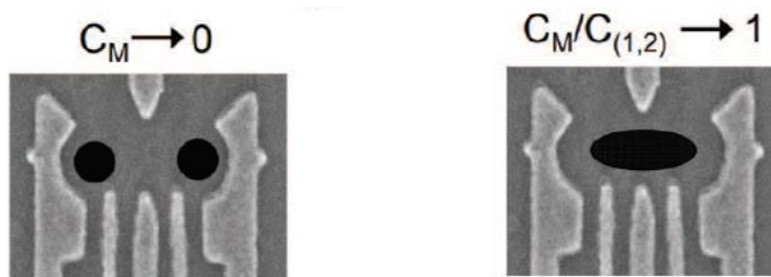
Figure 1.3.3 Weakly (left) and strongly (right) coupled quantum dots.
