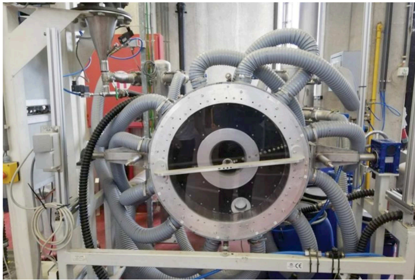
Figure 1.4: Vortex reactor technology developed in Ghent university used for pyrolysis step in gasification [8].
