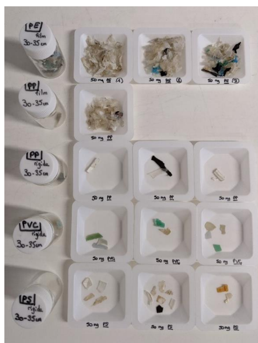
Fig. S 1: Particles in 50 mg aliquot in triplicates for PE films, PP films, PP fragments, PVC fragments and PS fragments
