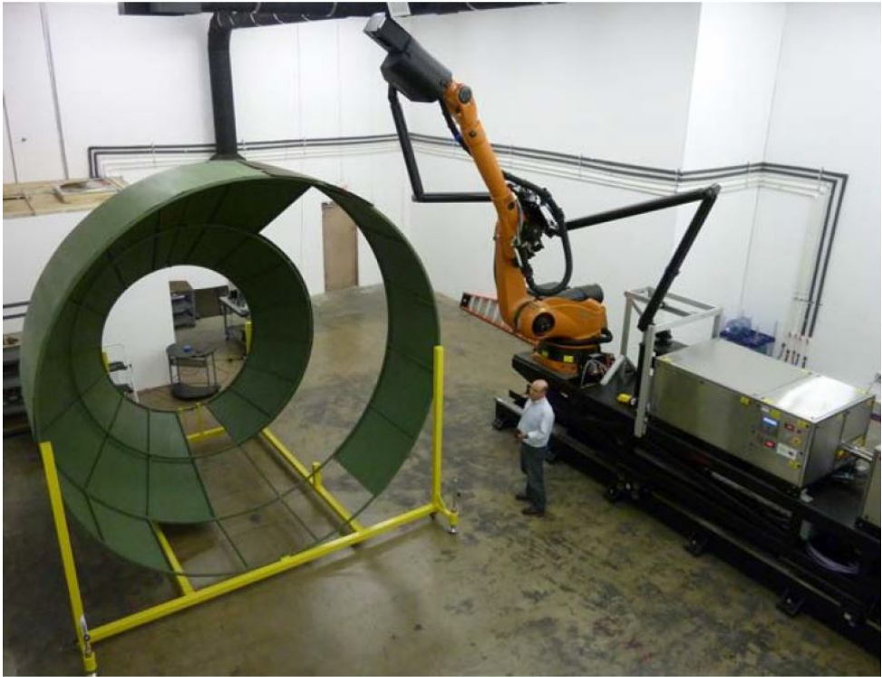
Figure 1.11 – LUCIE - a flexible system for the laser ultrasonic testing of large-scale parts of planes (reprinted from Ref. [56]).
