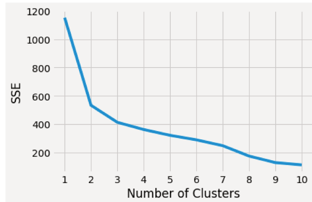
FIGURE 4.3: SSE for K-means algorithm for the second model
