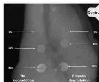
Fig. 5 Ex vivo X-ray images of non-degraded (left-hand side) and degraded (right-hand side) PCL-TIB/PLA 50 - b -PEG- b -PLA 50 blends sample plates implanted in a 4 cm thick anatomical model. Control corresponds to 2 mm thick aluminum wedge. Percentages correspond to iodine weight ratios.
