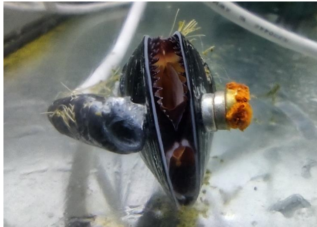
Figure 9: Valvometry device on a mussel. On the left a hall captor was glued and on the right magnets. Difference of potential is varying in function of the valve movements.
