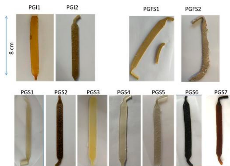
Figure 3. Photographs of elastomer sheets obtained by extrusion of their prepolymers when driven by the twin screws at a speed of 200 rpm and heated at 180 °C.
