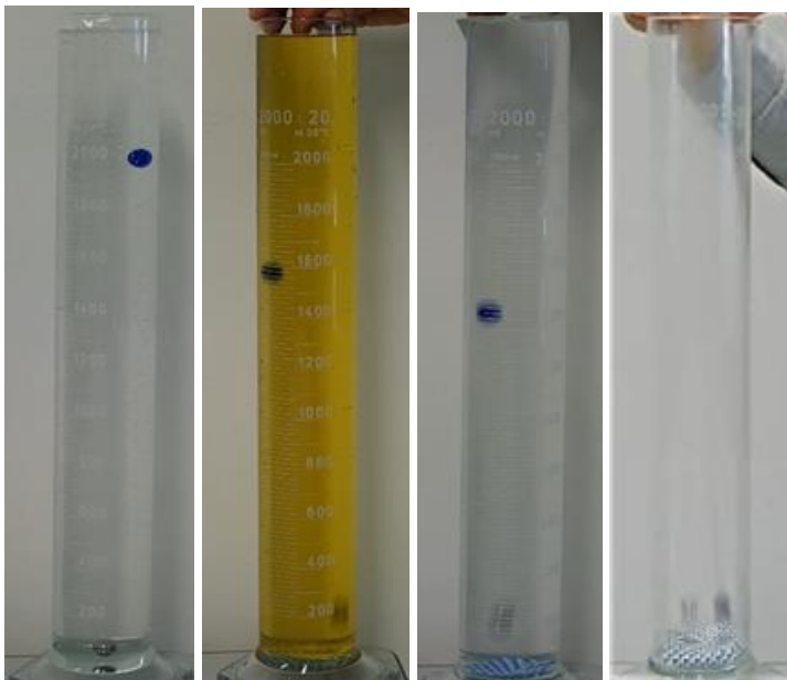
Fig. 4.3 The fall of two little balls in glycerine, in oil, in water and in air. Source: my experiment images.
