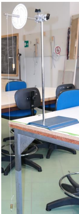
Fig. 4.1. A comparison of the oscillation time of two pendulums, one 4 times longer than the other. Source: my photo of the experiment.
