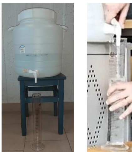
Fig. 4.2. Our water clock had to keep the height of the liquid in the tank steady and the tap had to be fully open to achieve a constant flow of water over time. Source: my photos of the experiment.
