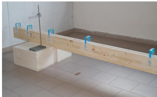
Fig. 4.12. The inclined plane with the bells and the pendulum used to verify the law of odd numbers. Source: my own experiment image.
