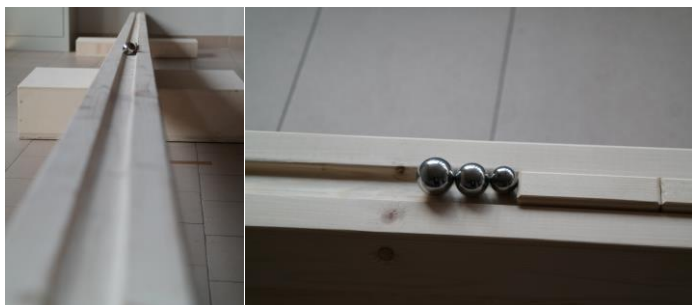
Fig. 4.11. The groove and the balls used. Source: my own experiment images.
