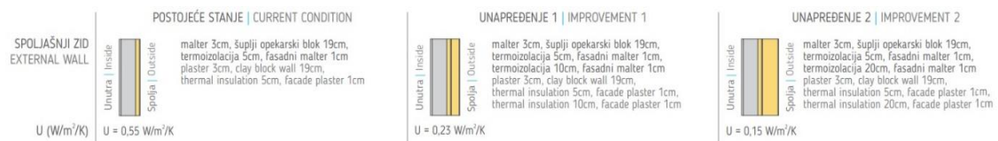
Figure 39. Energy performance improvement for external wall of residential buildings for apartment blocks in BIH made at the end of XX and beginning of the XXI century (Arnautovic-Aksic et al. 2016)
