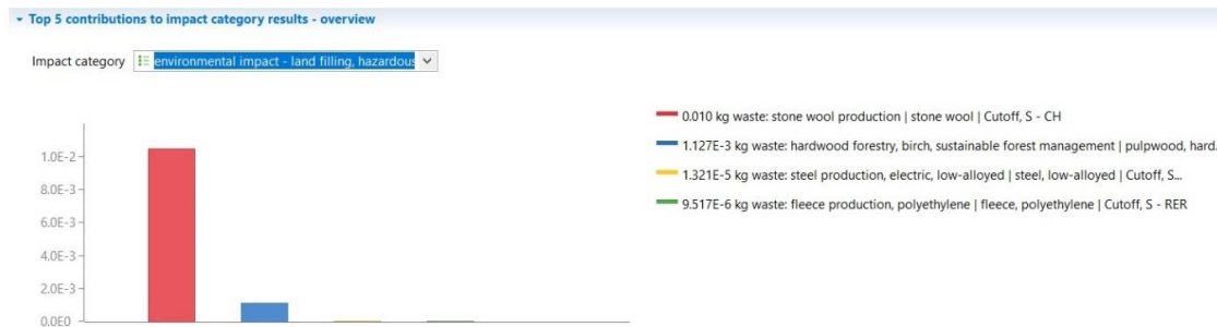
Figure 149. The environmental impact in terms of land filling - hazardous waste, calculated in the OpenLCA 1.10.1. tool
