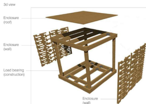
Figure 22. Picture of the Pixel in the exhibition in Mostar 2015 (left) and exploded 3D model of the wooden structure (right)
