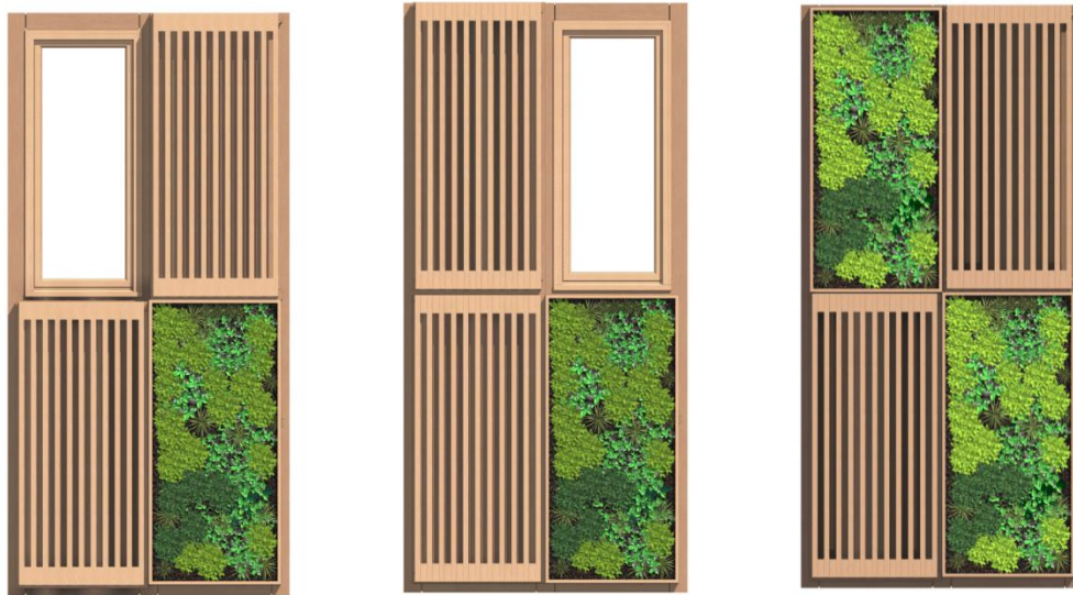
Figure 95. First position of the window (left), second position of the window (middle) and wall without the window (right)
