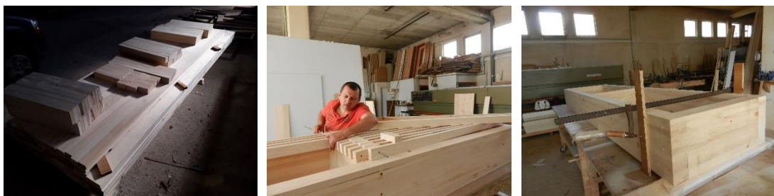
Figure 69. Picture of the GDC wall prototype made in Herzegovina. Picture left – wooden parts cut and ready to be laminated, middle – wooden slats assembly, right – wooden structure/frame. (photo Androšević)
