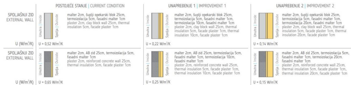
Figure 36. Energy performance improvement for external wall of residential buildings for single-family houses in BIH made at the end of XX and beginning of the XXI century (Arnautovic-Aksic et al. 2016)
