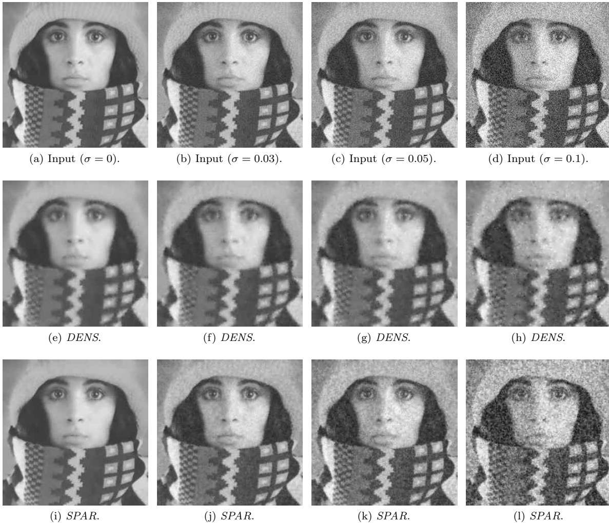
Figure 2.6: Reconstruction with the sparsification and densification methods with 10% of total pixels saved.
