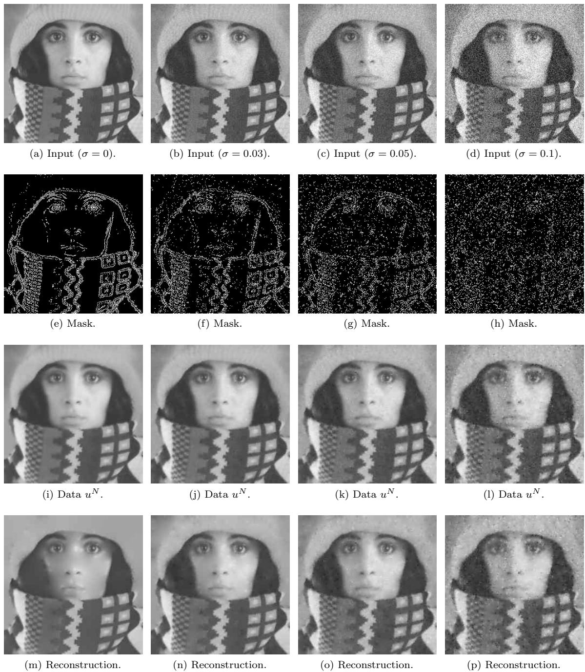
Figure 2.7: Reconstruction with L_2 -INC-T-E method with 10% of total pixels saved.
