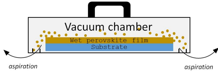
Figure II-10: a. Photo of the vacuum chamber used for the solvent extraction of wet perovskite layer after the slot-die deposition. b. Schematic description of the vacuum aspiration method.
