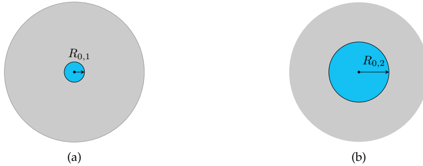
Figure 5.24: Initial slight opening (in blue) in the wall at the interface (in gray) for (a) an initial contact radius R_{0,1} = 14 mm and (b) an initial contact radius R_{0,2} = 42 mm.
