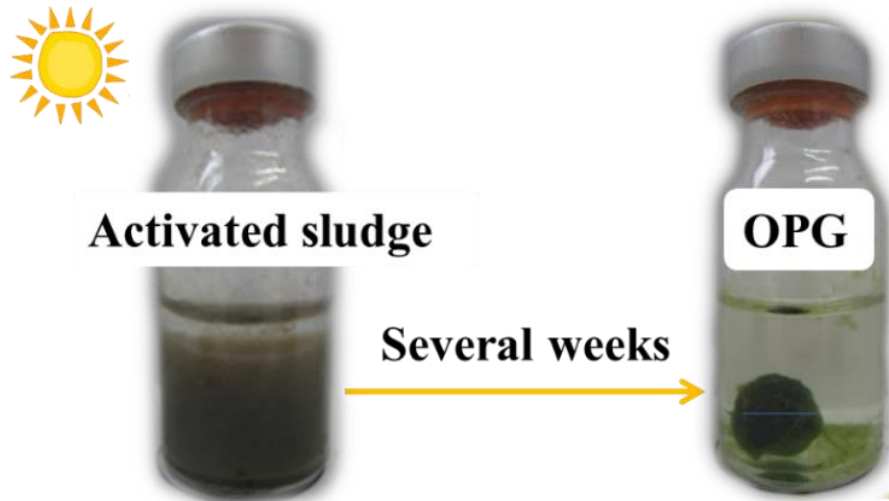
Figure I.2 Photogranulation of activated sludge under static conditions (vial diameter is 2.5 cm).
