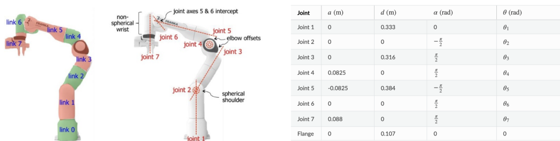
Figure 2.2: Geometric representation of the manipulator Franka Emika Panda and its associated Denavit-Hartenberg parameters.
