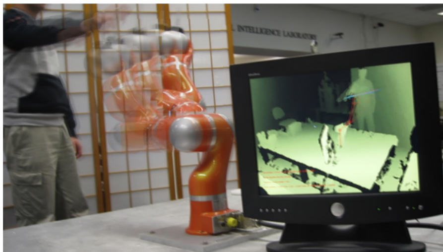
Figure 3.2: Human-robot collision avoidance in depth space with potential field method.
