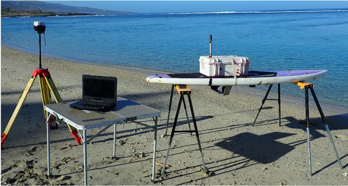
(a) ASV preparation for a survey in remote mode with the mobile GPS RTK base station (on the yellow tripod)
