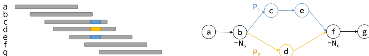
Figure 3.5 – A bubble in a similarity graph. Bubbles are caused either by errors or by true variant in reads. One can rely on the coverage information of such reads to assess whether it is a variant or an error (not illustrated in this figure). They cause alternative paths in the graph, and thus can be removed to gain contiguity, or kept to gain knowledge on variants.
