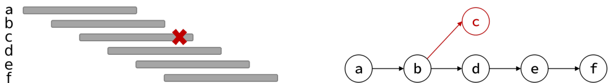
Figure 3.4 – A tip in a similarity graph. Considering a set of overlapping reads, with one ( c ) having enough errors to miss an expected connection to the d , e and f reads. This configuration leads a tip in the similarity graph, that has to be removed.
