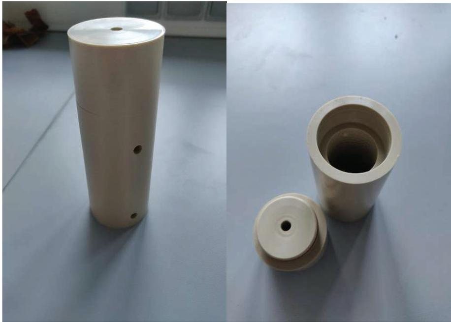
Figure 32. Cylindrical cell for VOC measurement
