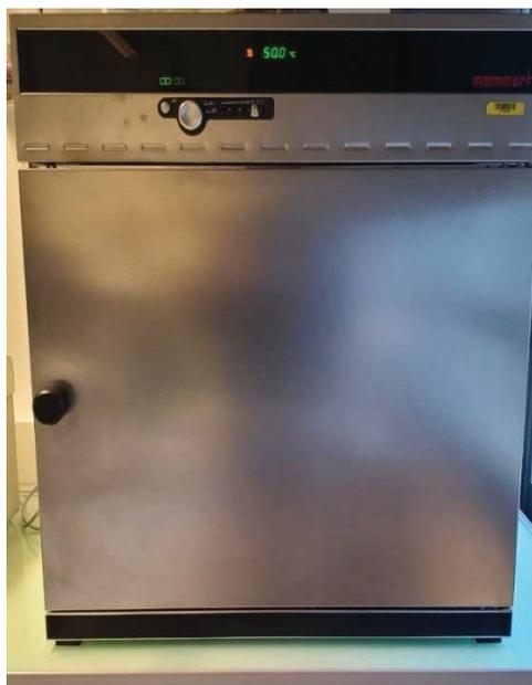
S 10. Furnace for baking electrodeposited chitosan chip
