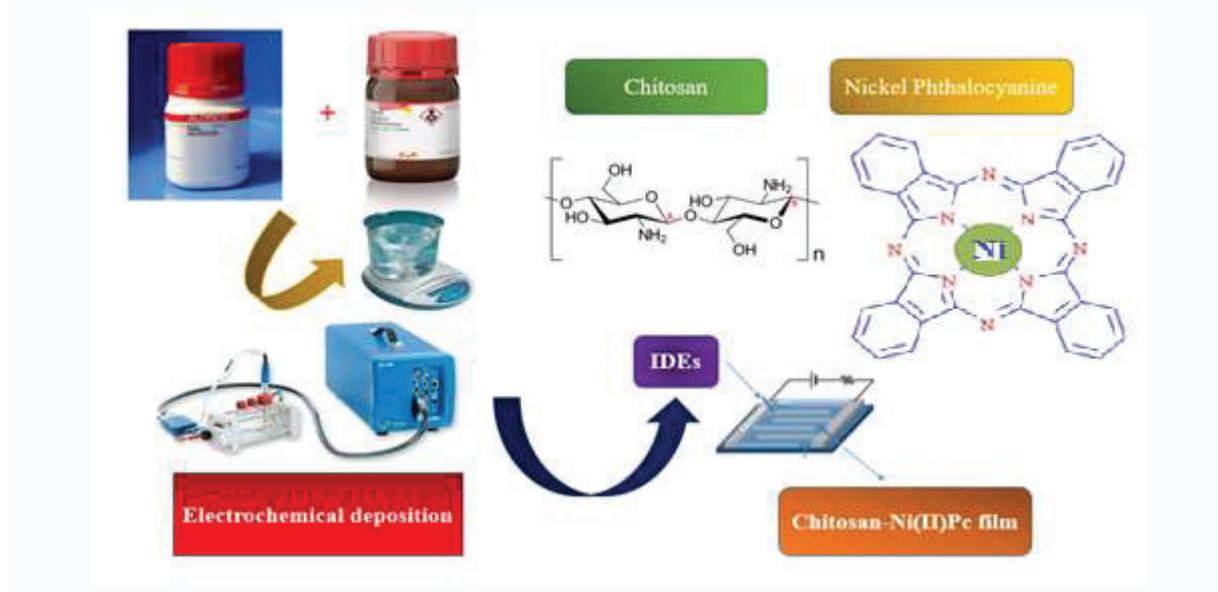
Figure 9. Chitosan-Nickel-phthalocyanine composites formation for gas sensing ability
