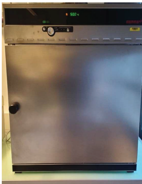
S 10. Furnace for baking electrodeposited chitosan chip
