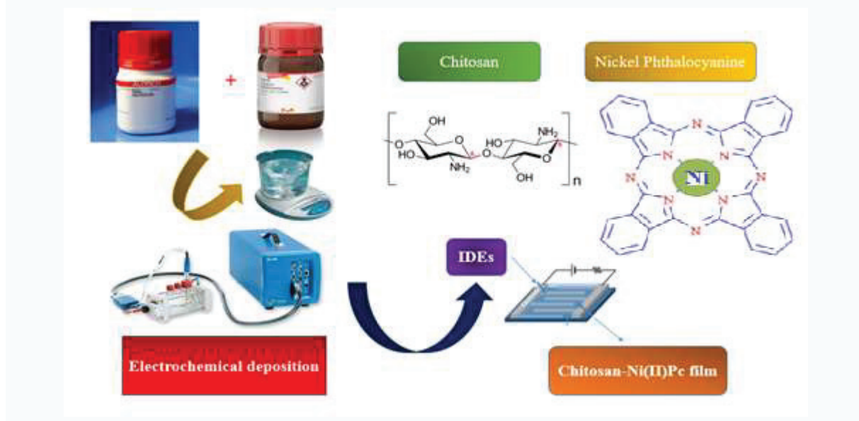
Figure 9. Chitosan-Nickel-phthalocyanine composites formation for gas sensing ability
