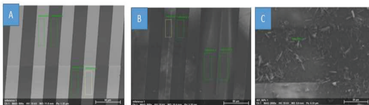
S 12. SEM Image of (a) bare chip, (b) chitosan deposited on chip and (c) Chitosan doped NiPc deposited on chip
