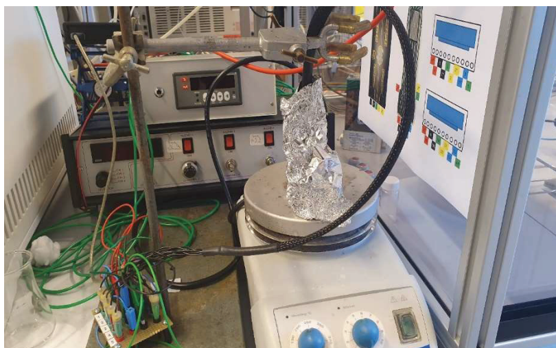
S 4. Conductivity measurements of KCl solution using interdigitated electrodes
