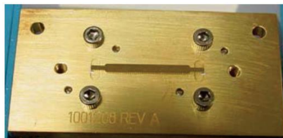
Figure 2.15: Fabricated array installed in a brass test fixture with two WR-3 waveguide [29].
