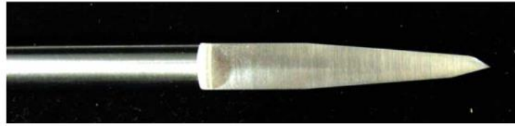
Figure 2.2: The high-speed steel machine tool used for the fabrication of the 230 GHz drilled horn prototype [15].
