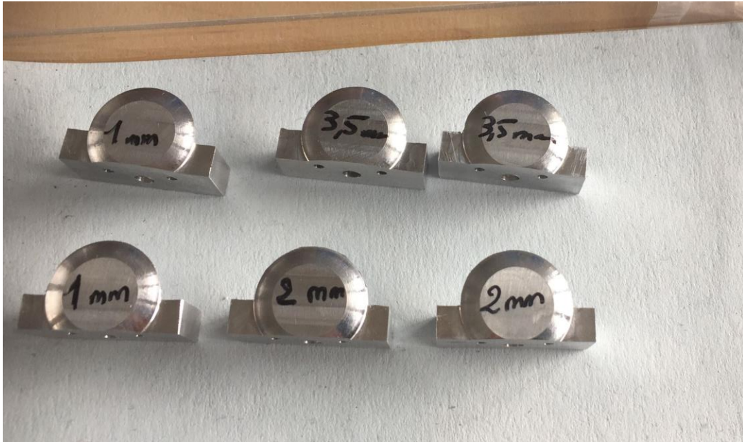
Figure 7.36: The prototypes of the metallic flare with different thicknesses.
