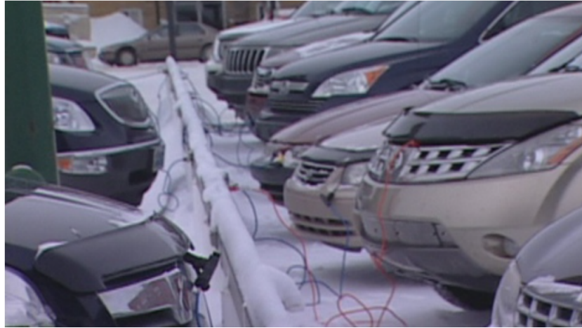
FIGURE 3.2 – Example of block heaters in a parking lot.
