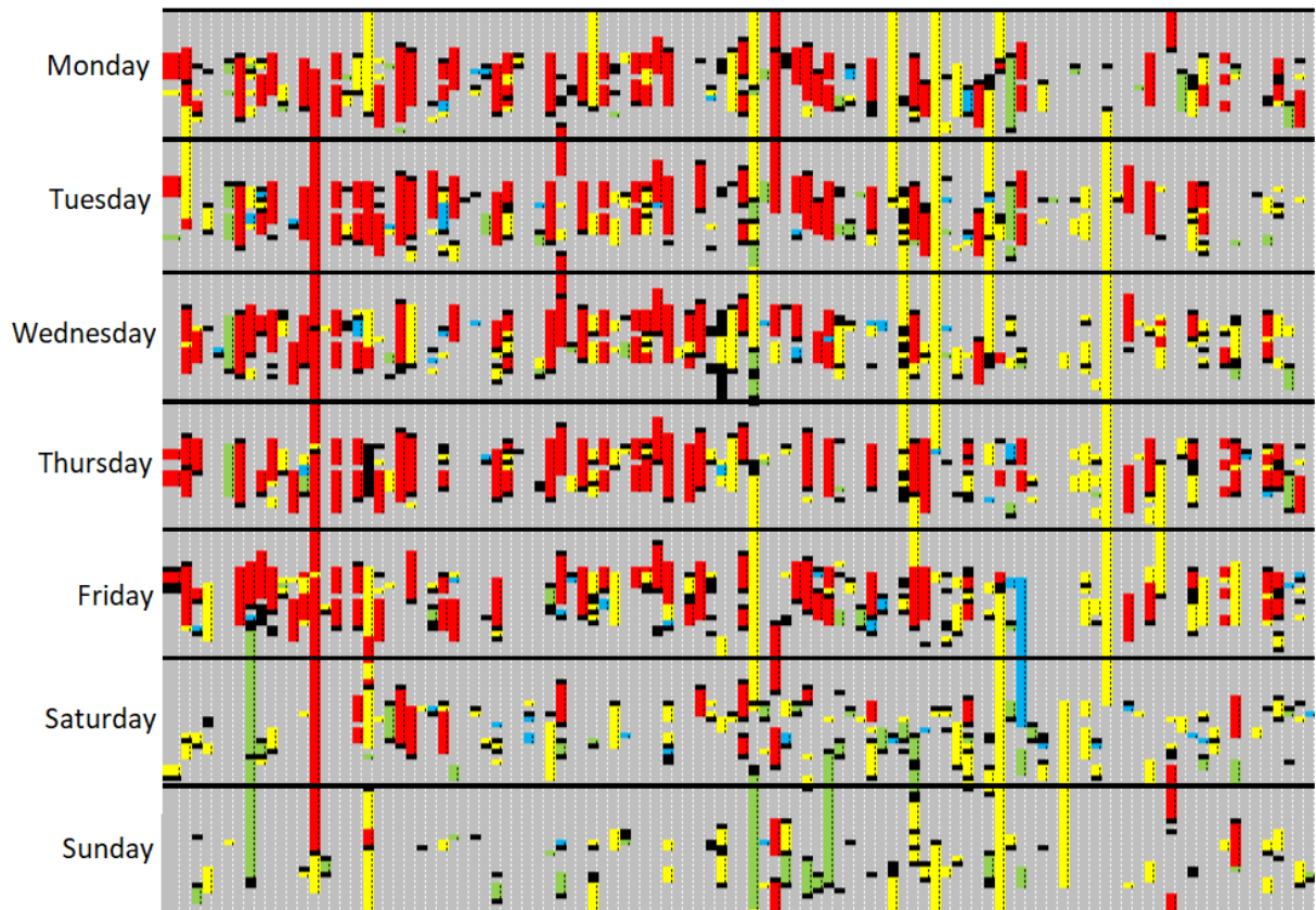
FIGURE 3.13 – An example of the presence schedule of 107 EV during one week (each EV is a vertical colored line). Black cells represent EV is the middle of a trip, gray cells at home, red cells at workplace, blue cells at stores, green cells visiting family or friends and yellow ones represent the rest of possible locations.
