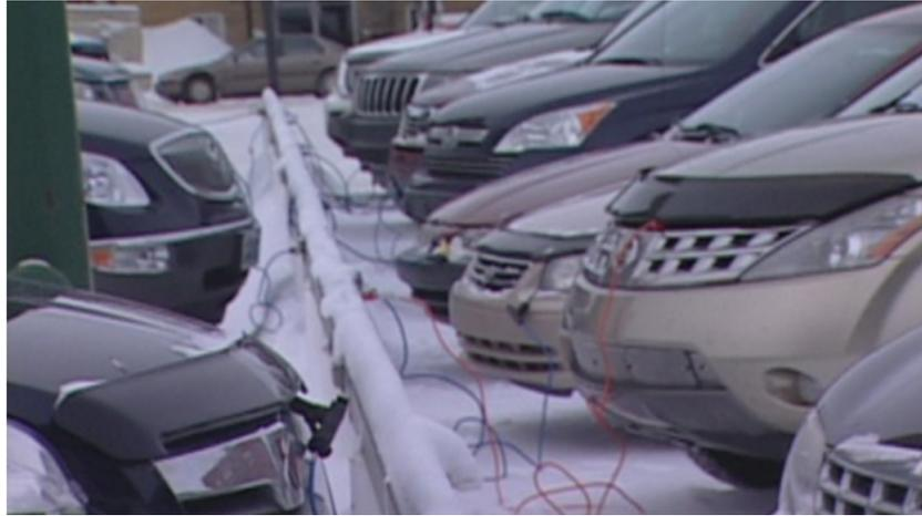
FIGURE 3.2 – Example of block heaters in a parking lot.
