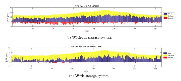
FIGURE 2.4 – Example of the daily electricity production during one year with 15MW of REn installed capacity with a distribution of 75% PV and 25% wind power. Unit : kWh/inhabitant.
