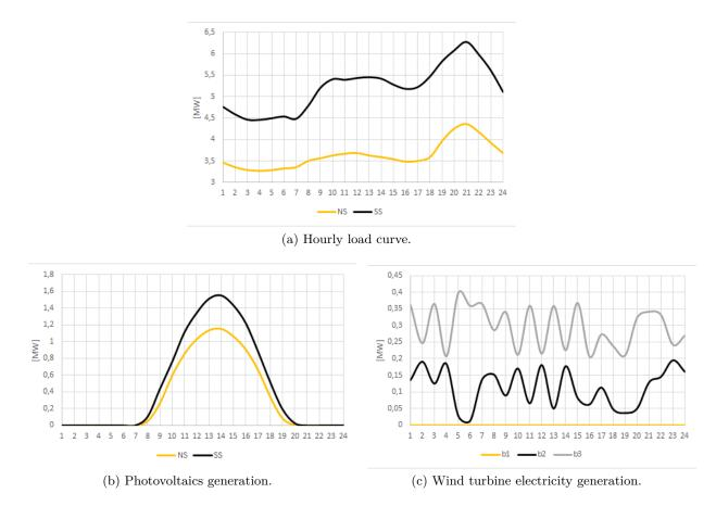
FIGURE 2.6 – Parameters of electricity generation from REn by hour used for the optimization model for normal season (NS) and summer season (SS). Unit : MW.
