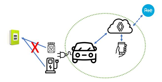
FIGURE 3.22 – Proposed communication diagram between EV and the carmaker's cloud taking public data from DSO/TSO about the electricity consumption. Source : authors.
