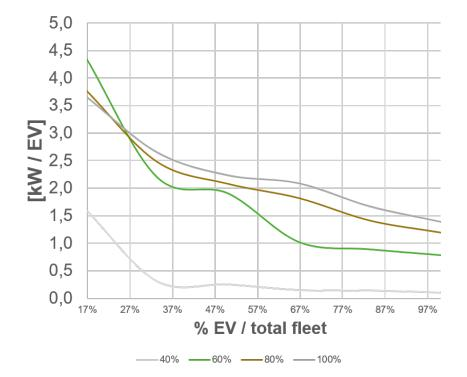
FIGURE 2.10 – Maximal discharge power for different REn shares and different EV fleets. Unit : kW/EV. Source : authors.
