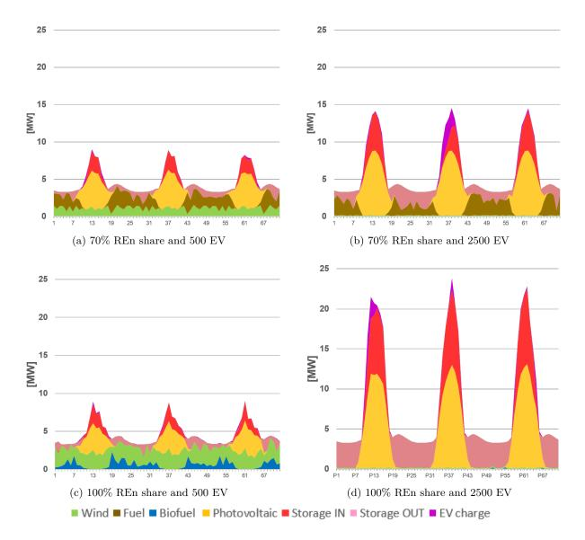
FIGURE 2.13 – Power system behavior in one hour time step during 3 days (72 hours). Unit : MW. Source : authors.
