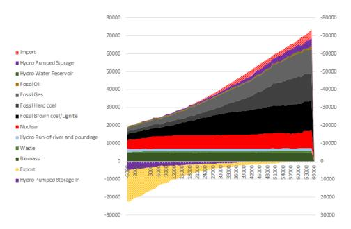
FIGURE 4.6 – Electricity generation by power plant type as function of residual demand. Unit : MW. Source : authors with original data from ENTSOE.
