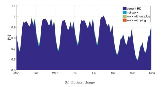
FIGURE 3.15 – Natural and optimal charge comparison for a week of summer in 2019. 10% of EV with the electricity mix as it is today.
