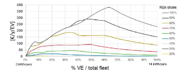
FIGURE 2.8 – Saving for the power system for different REn shares and different EV fleets (including running costs and investment costs) from the optimization model. Unit :  $\in$ /y/EV. Source : authors.
