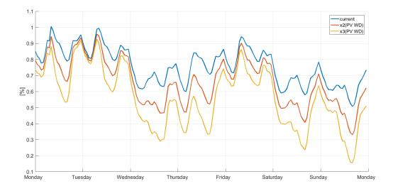
FIGURE 3.6 – Residual demand in France normalized with respect to the average value, for one week in spring. The blue curve is the original one. The red one is the resulting curve of doubling the PV and wind installed capacities and the orange curve is the resulting curve of triplicating these capacities.
