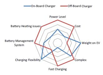
FIGURE 3.4 – Comparison between On-board and Off-board chargers. Source : [Ashfaq, 2021].
