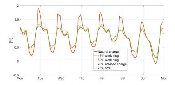
FIGURE 3.18 – Evolution of the residual demand curve from natural charge to optimal charge improving the most impacting parameters until the application of V2G for one same week of summer in France. With 7 times the current PV installed capacity, 4 times the wind power and 70% of EV.
