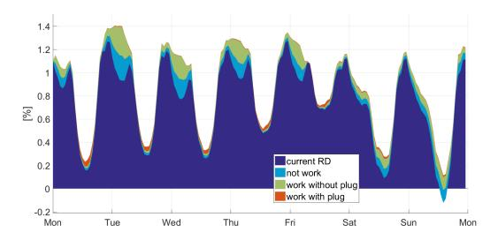
peak hours passes from an amplitude of 189% to 126% with respect to the average value (100%).
