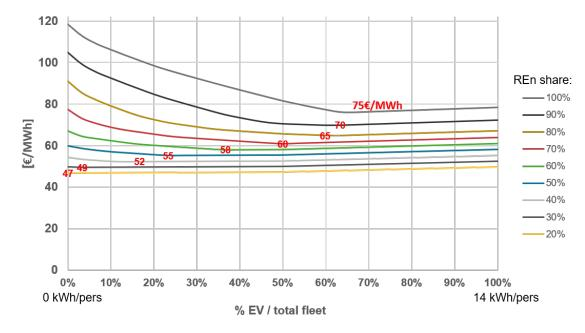
FIGURE 2.7 – For different REn shares and different EV fleets (including running costs and investment costs) from the optimization model. Average cost per MWh. Unit : €/MWh. Source : authors.
