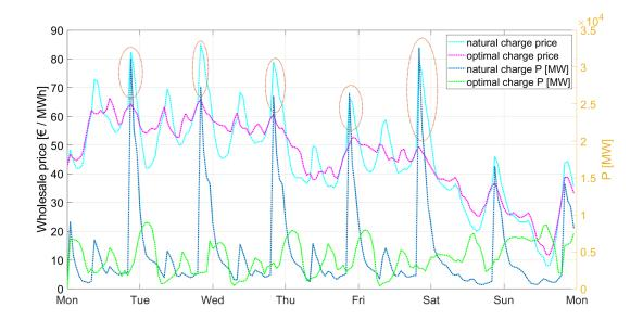
FIGURE 4.8 – Results for a random week of charge powers and electricity prices in natural and in optimal charge. Left unit : €/MWh. Right unit : MW. Source : authors.
