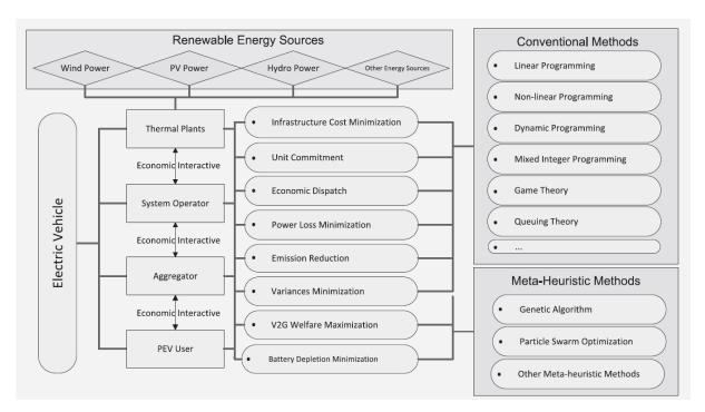
FIGURE 3.8 – Smart charging objectives and methods. Source : [Yang, 2015].
