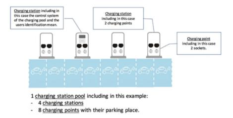
FIGURE 3.1 – Illustration of the components of the recharging infrastructure. Source : AFIREV.
