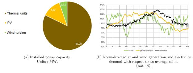
FIGURE 2.1 – Porto Santo's power system and weather characteristics. Source : Authors with data from EEM.
