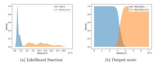
Figure 3.37: (a) Likelihood function and (b) output score of a binary Naive Bayes classifier using KDE for a new voltage sag signature  $q^*$  to the class  $C_2$ , given the distance to the class  $x = d_2(q^*)$ .
