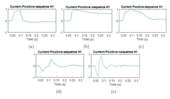
Figure 3.20: Current positive-sequence harmonic 1: (a) downstream fault, (b) downstream transformer energizing, (c) downstream motor startup (d) upstream fault and (e) upstream transformer energizing
