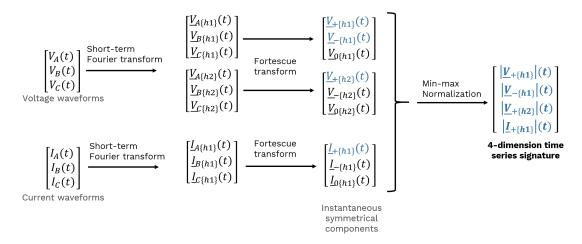
Figure 3.12: Feature extraction process and the obtained components.
