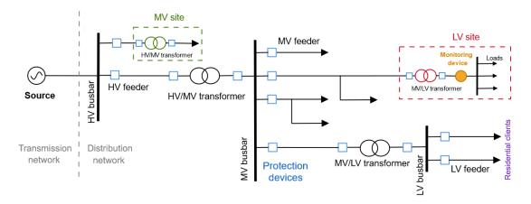
Figure 1.1: Simplified diagram of a distribution network. The monitoring device at a LV industrial site is illustrated.
