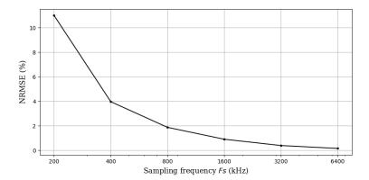
Figure 3.11: RMSE (%) as a function of the sampling frequency of the electrical waveforms
