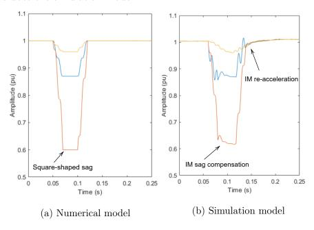
Figure 2.3: RMS values of a synthetic voltage sag generated with a numerical model (a) and a simulation model (b). Only the simulation model emulates the influence of the induction motor (IM) on the sag.
