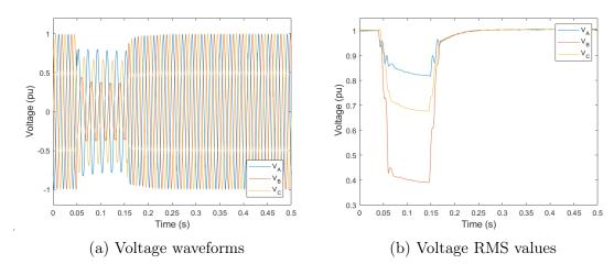
Figure 1.3: Voltage sag representations of a double-phase fault
