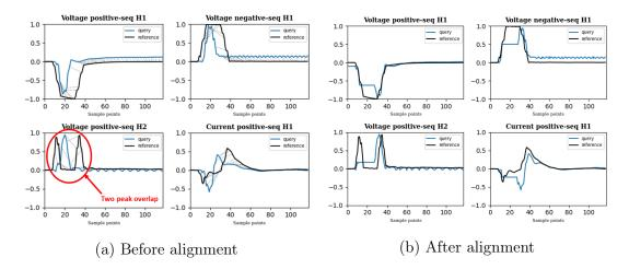
Figure 4.12: Classification errors in experiment no. 3. Reference signature of class A2 (50 ms) and query signature of class A2 (30 ms)
