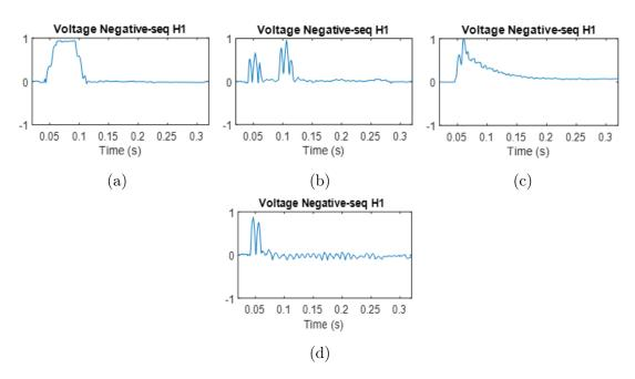
Figure 3.18: Voltage negative-sequence harmonic 1: (a) unbalanced fault, (b) balanced fault, (c) transformer energizing and (d) motor startup
