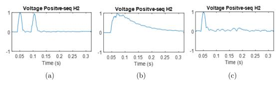
Figure 3.19: Voltage positive-sequence harmonic 2: (a) fault, (b) transformer energizing, (c) motor direct startup
