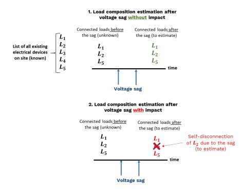
Figure 5.2: Two-step approach for load composition estimation after a voltage sag with and without impact
