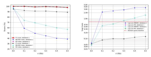
(a) F1-score and mean values for NB-KDE (b) Log-loss values for NB-KDE and RD and RD confidence indexes confidence indexes
