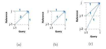
Figure 3.26: Local step patterns: (a) symmetric2, (b) symmetric1, (c) asymmetric
