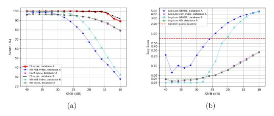
Figure 4.4: Centroid estimation method: (a) F1-score and mean values for NB-KDE and RD indexes and the corresponding (b) Log-loss values associated to the output predictions for 16 different noise levels.
