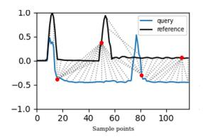
Figure 3.24: Poor time alignment due to singularity points (red) can lead to high distortion of time series.
