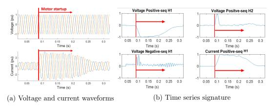
Figure 3.15: Voltage sag caused by a downstream induction motor startup (field data).
