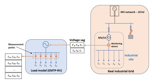
Figure 5.3: Diagram of the load model used for the load composition estimation during a voltage sag
