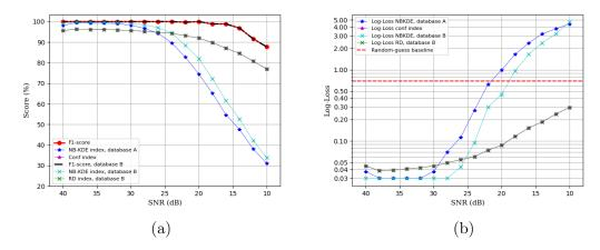
Figure 4.3: Bootstrapping method: (a) F1-score and mean values for NB-KDE and RD indexes and the corresponding (b) Log-loss values associated to the output predictions for 16 different noise levels.
