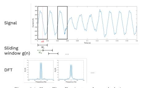
Figure 3.4: Short-Time Fourier transform calculation
