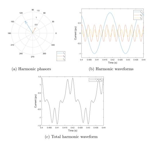
Figure 1.8: Harmonic distortion of current and decomposition in harmonic components
