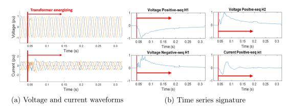
Figure 3.14: Voltage sag caused by an upstream transformer energizing (field data).
