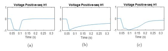
Figure 3.17: Voltage positive-sequence harmonic 1: (a) fault, (b) transformer energizing and (c) motor startup
