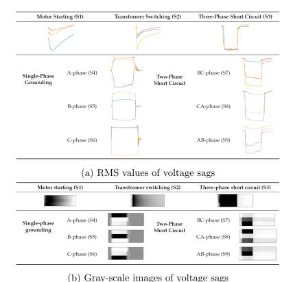
Figure 2.4: Format transformation from voltage waveforms to (a) RMS values and (b) and gray-scale images, for voltage sag source identification based on image processing techniques. [2].
