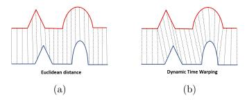
Figure 3.21: Time series matching using (a) Euclidean distance and (b) Dynamic Time Warping algorithm.
