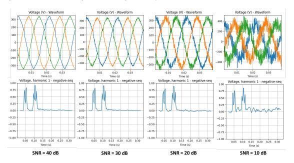
Figure 4.5: Varying noise levels on the voltage waveform and their impact to the signatures
