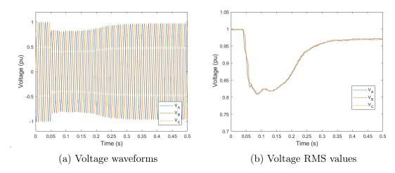
Figure 1.5: Voltage sag representations due to an induction motor direct startup
