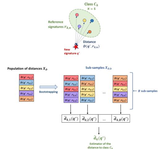
Figure 3.32: Calculation of the distance to a class  $C_k$  using bootstrapping
