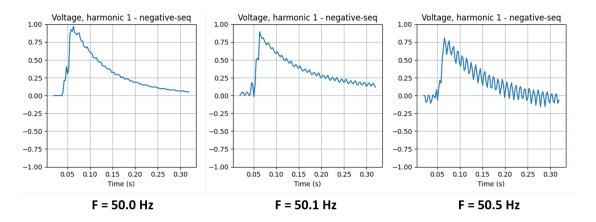
Figure 4.8: Effects of the fundamental frequency variations on the second ISC of a voltage sag caused by a transformer energizing.
