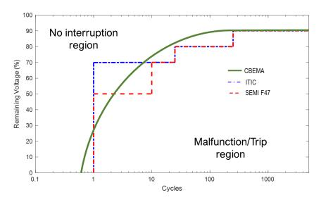
Figure 1.6: CBEMA, ITIC and SEMI F47 curves, from [1]
