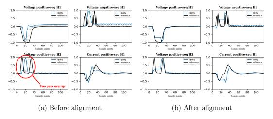
Figure 4.11: Classification errors in experiment no. 3. Reference signature of class A1 (50 ms) and query signature of class A2 (30 ms)
