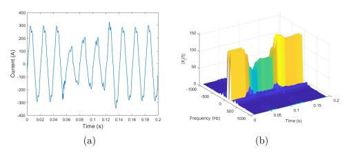
Figure 3.7: One-phase current signal (a) and the module of its corresponding Short-Time Fourier Transform (b).
