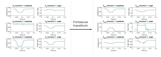
Figure 3.9: Fortescue transform applied to three-phase voltage time series (harmonic 1 or fundamental), resulting in three instantaneous symmetrical components
