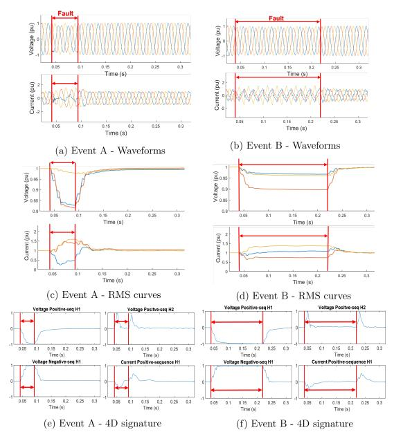
Figure 3.16: Two voltage sags caused by upstream unbalanced faults (A2)
