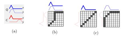
Figure 3.23: Time alignment of (a) two multivariate time series with (b) Dependent DTW and (c) Independent DTW [3].
