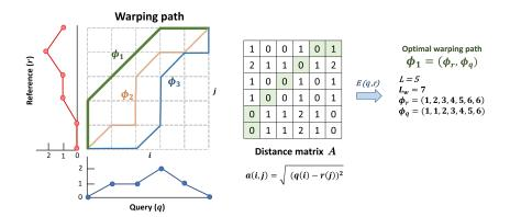
Figure 3.22: Time alignment of two univariate time series. The optimal warping path is given by the lowest value of the cumulative cost E, obtained from the distance matrix A.
