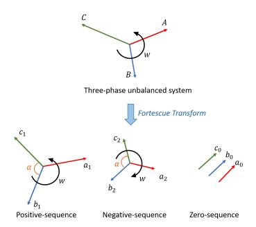
Figure 3.8: Fortescue transform applied to a three-phase unbalanced system.
