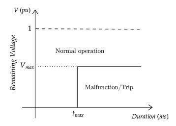
Figure 1.7: Voltage-tolerance curve (VTC)
