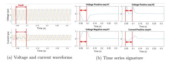
Figure 3.13: Voltage sag caused by an upstream unbalanced fault (field data).
