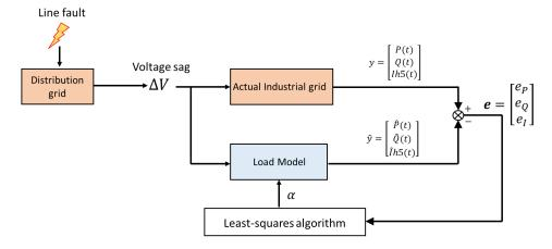
Figure 5.4: Measurement-based approach for load composition estimation
