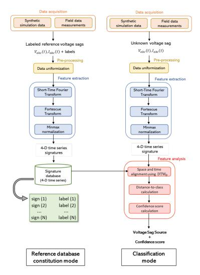
Figure 3.1: Flowchart of the two modes: reference database constitution and classification
