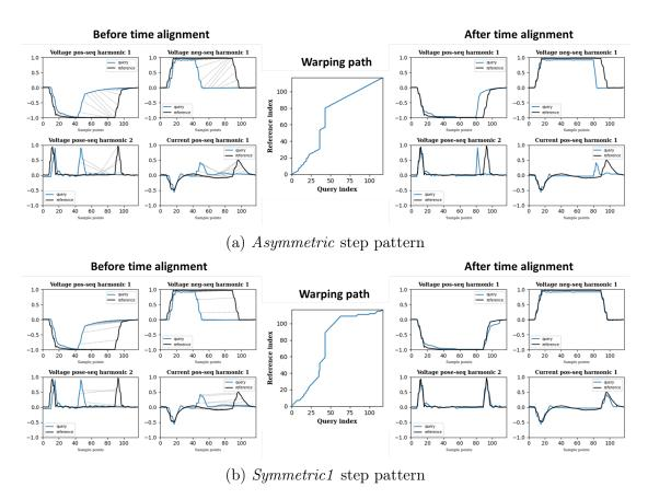
Figure 3.29: Time alignment results of two signatures belonging to the same class, using (a) asymmetric and (b) symmetric1 step patterns.
