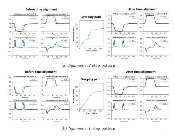
Figure 3.27: Time alignment results of two signatures of the same class, using (a) symmetric2 and (b) symmetric1 step patterns.
