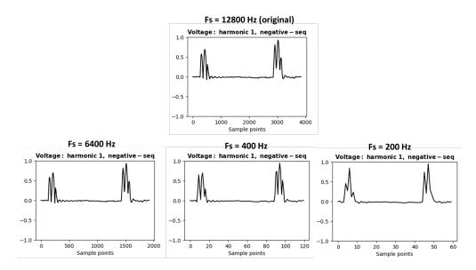
Figure 3.10: Waveform downsampling effect on the extracted signatures
