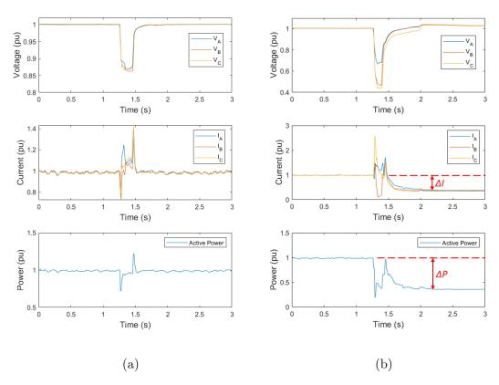
Figure 5.1: (a) Voltage sag without impact and (b) voltage sag with load self-disconnection or load tripping
