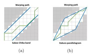
Figure 3.25: Global constraints on the warping path (a) Sakoe-Chiba band and (b) Itakura parallelogram
