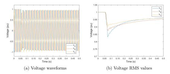
Figure 1.4: Voltage sag representations due to a transformer energizing
