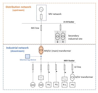
Figure 3.3: Simplified diagram of the simulated industrial network.
