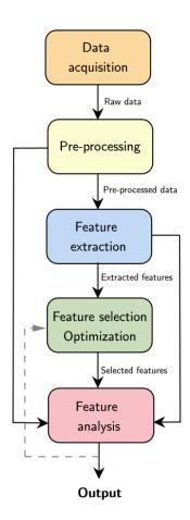
Figure 2.2: Generalized flowchart for power quality disturbance classification
