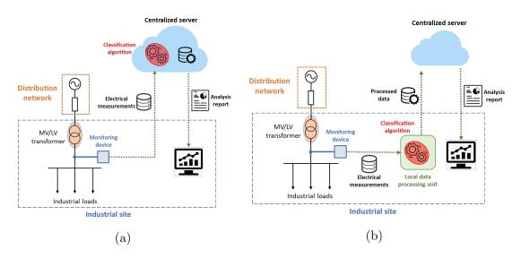
Figure 3.2: (a) Centralized and (b) decentralized approaches for data collection and processing
