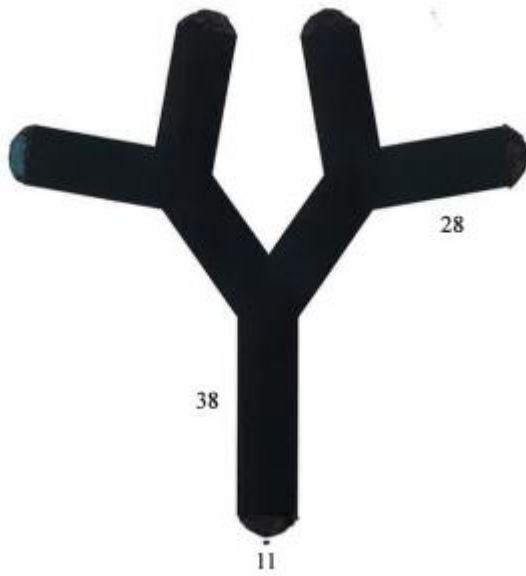
Figure 2: Real size artificial macroalgae unit Dictyota type. The measures are in mm.
