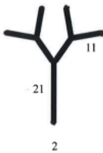
Figure 4: Real size artificial macroalgae unit turf type. The measures are in mm.
