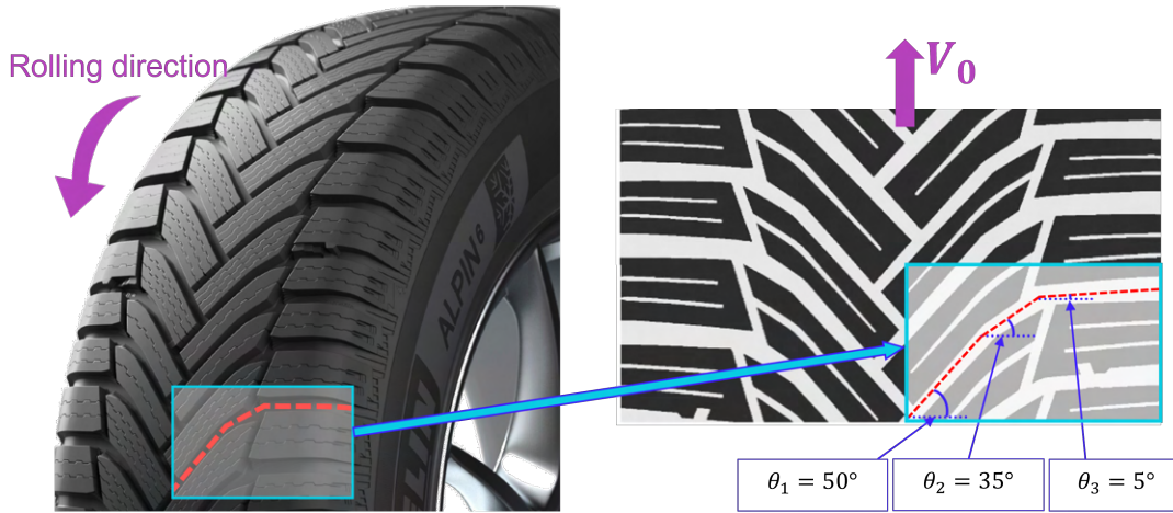
Figure 6.1 – Details of the Alpin 6 tread design with a highlight on a unique directional groove and its directions with respect to the horizontal axis.
