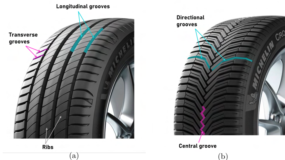
Figure 1.11 – Examples of 3D sculptures currently available on the market: MICHELIN Primacy 4 (a) and MICHELIN Cross Climate+ (b)
