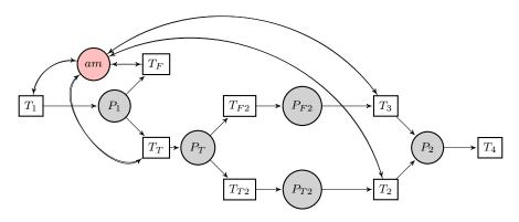
Figure 4.13: CPN sub-model of the withdraw() function in the Blind Auction contract
