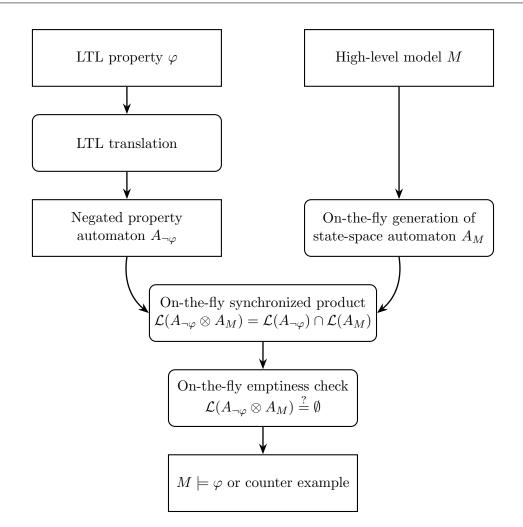
Figure 2.6: Automata-theoretic explicit LTL model checking
