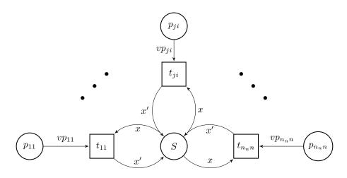
Figure 5.2: CPN model for a completely-free behavioural context
