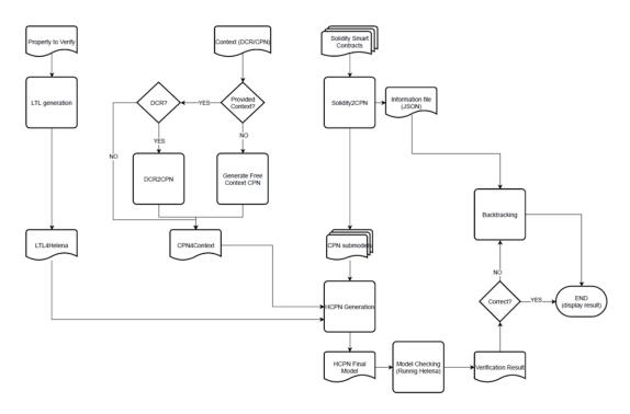
Figure 7.2: Architecture of the Solidity2CPN tool
