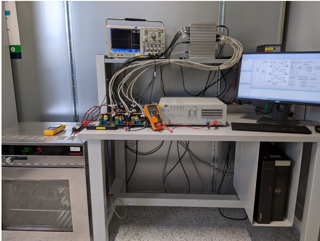
Fig. 4.24. Experimental setup of a small-scale prototype of modular converters with connected supercapacitors [32], [50]
