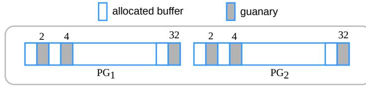
Figure 6.5: Bitmaps of SPP pages for a protection frequency  $F = 1$  and classes whose size is  $< 128B$ . 1 sub-page out of 2 is protected: all pages ( $PG_i$ ) have the same bitmap in the VMA.
