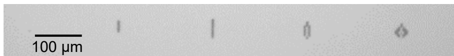
FIGURE 6.9: Ablation pattern along the propagation of the Bessel pen line with dz = 20 \mu\text{m} for single pulses and a pulse duration of 411 fs.
