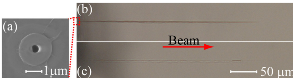
FIGURE 2.7: Electron microscope top view (a) and optical microscopy longitudinal cross sections (b,c) of void in fused silica after laser processing with Bessel beam. The continuous character is shown by filling with water (c) [Bhu+14]
