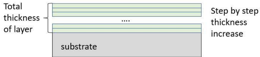
Figure 1-3. Schematic representation of dividing the layer into smaller sub layers of the same material.
