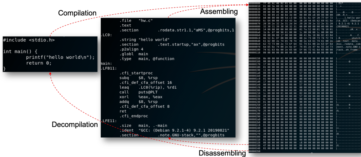
Figure 2.17 – [De]compilation and [de]assembling of a “hello word” code in C.
