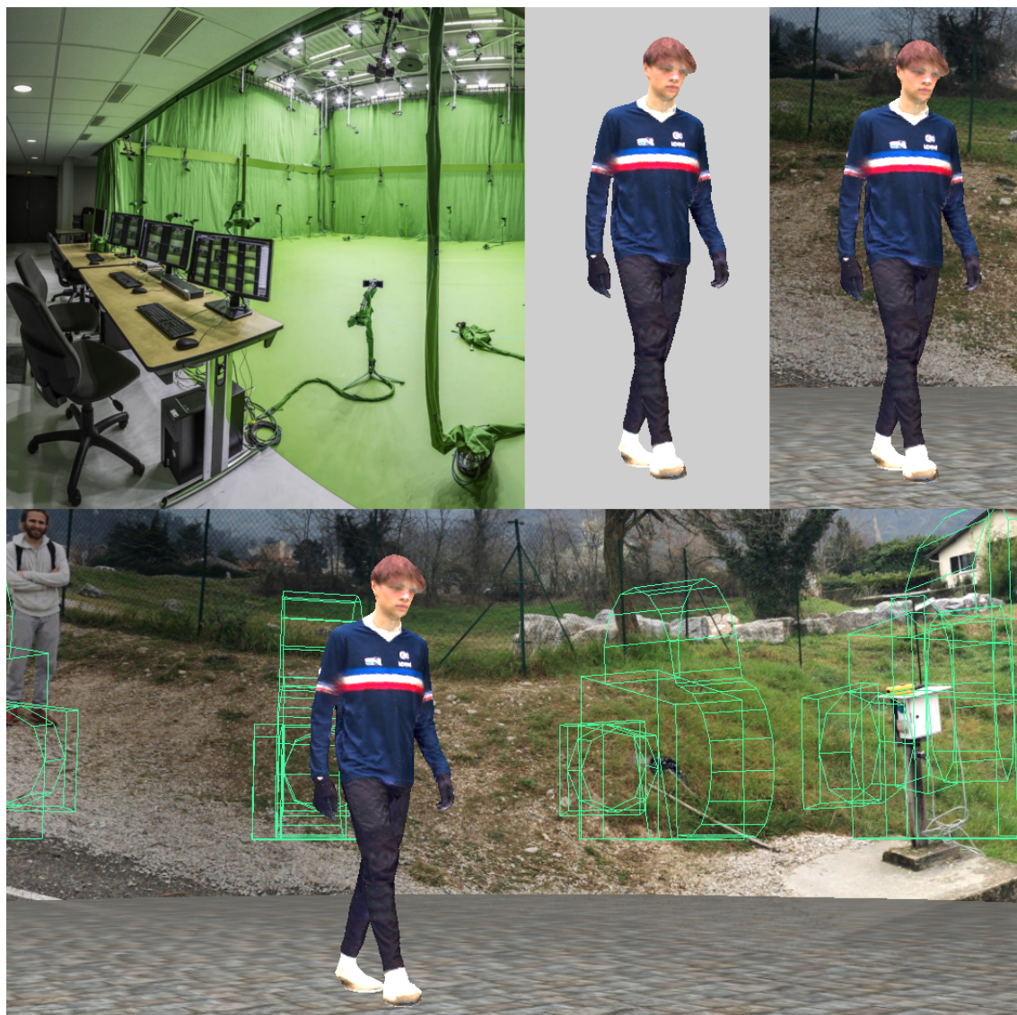
Figure 4.3: The Kinovis room allows for the capture of 3D textured meshes. These meshes are placed in a virtual environment, and then filmed from virtual cameras.
