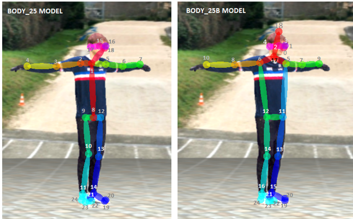
Figure 2.7: The body_25b OpenPose model is more accurate than the default body_25 one. As an example, the left knee is slightly misplaced on the default model. Keypoint definition and order also differ between both models.
