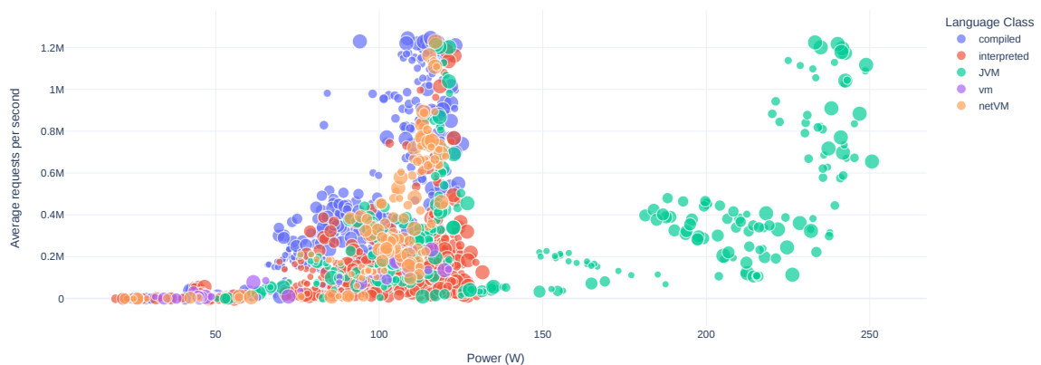
Figure 6.23: total request vs. average power consumption for JSON Serialization scenario (size of circles represents the number of clients)
