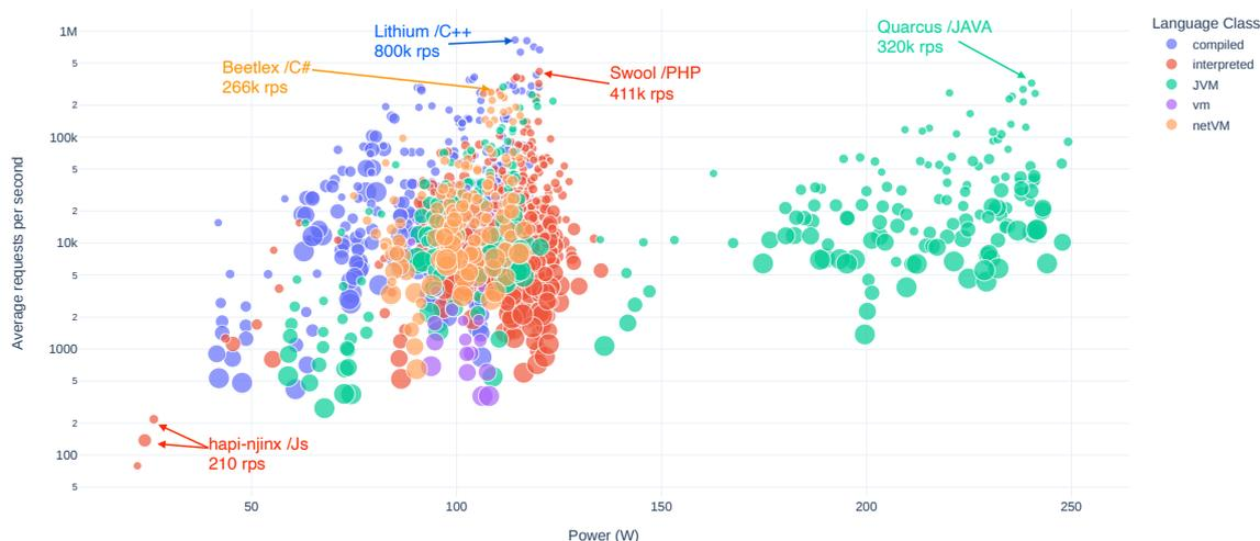
Figure 6.18: Total request vs. average power consumption for *multiple queries* scenario (size of circles represents the number of clients)
