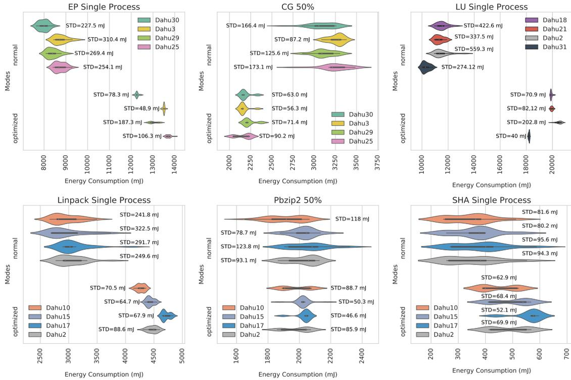
Figure 3.15: Energy variation comparison with/without applying our guidelines
