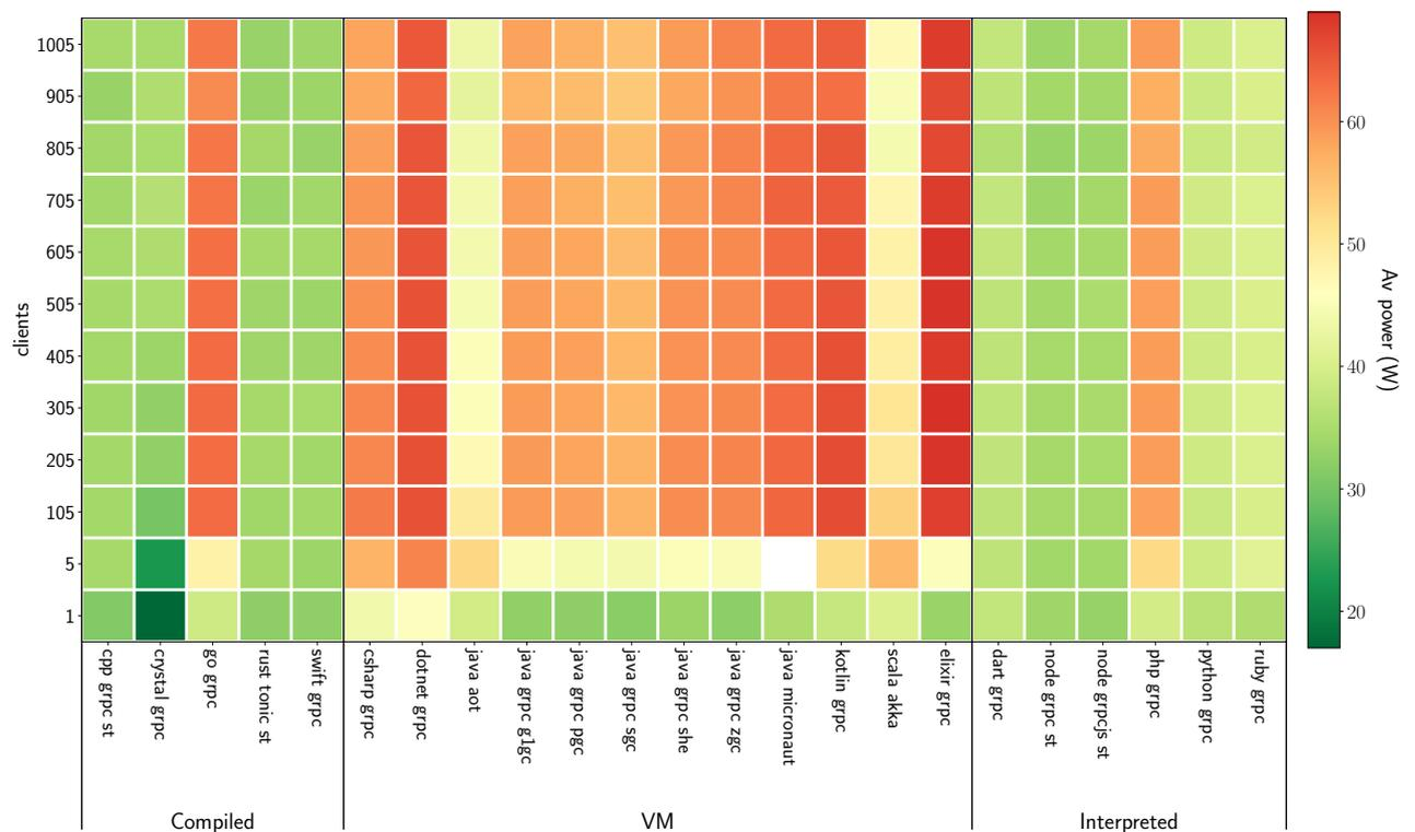
Figure 6.2: Average power consumption based on the number of the clients
