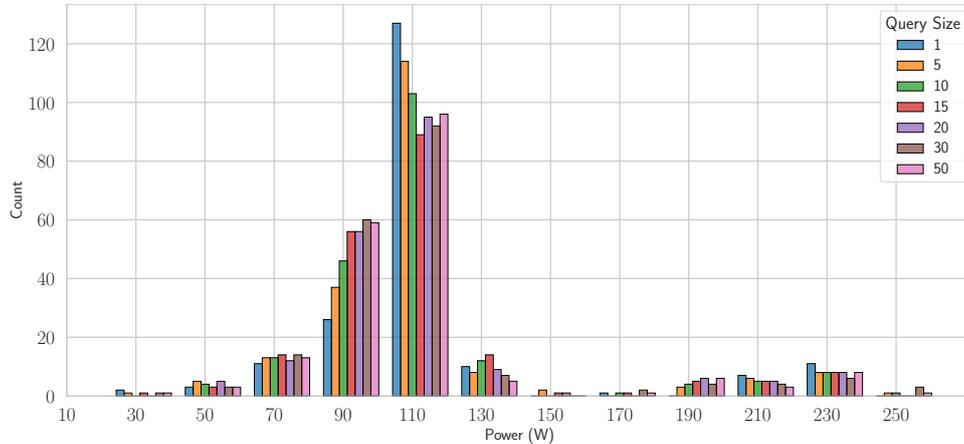
Figure 6.17: Distribution of average power consumption for the *multiple queries* scenario
