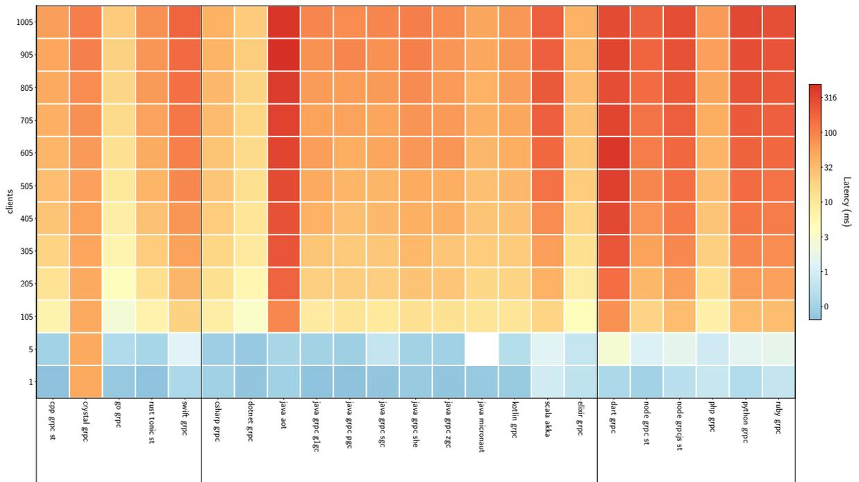
Figure 6.4: Tail latency (99%) based on the number of clients
