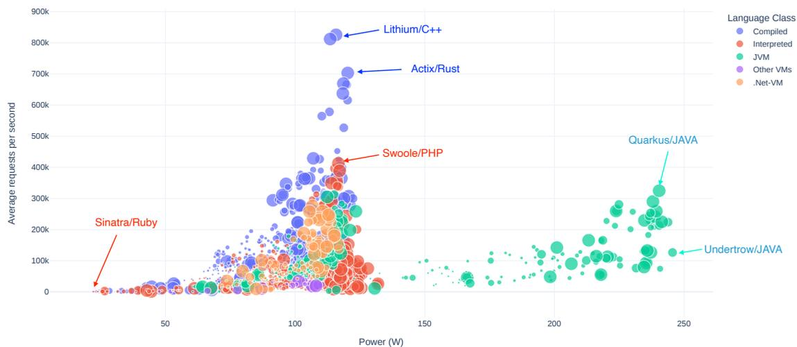
Figure 6.16: Total request vs. average power consumption for the *single query* scenario (size of circles represents the number of clients)
