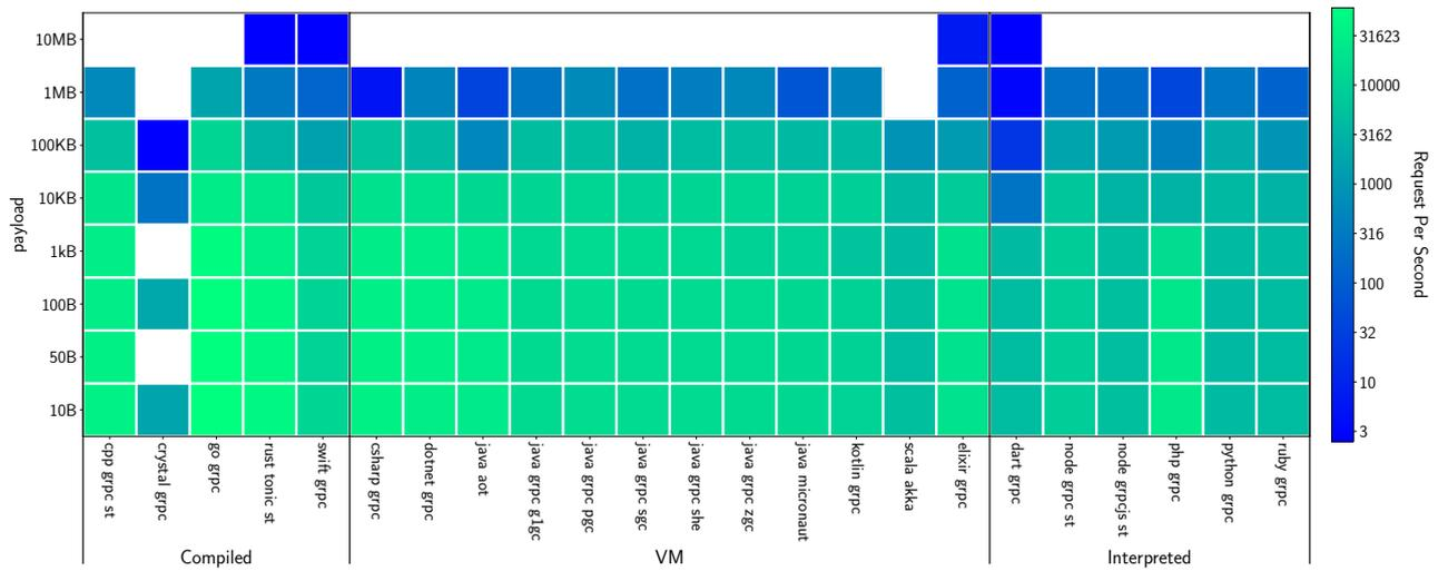
Figure 6.8: Number of requests per second based on the request size
