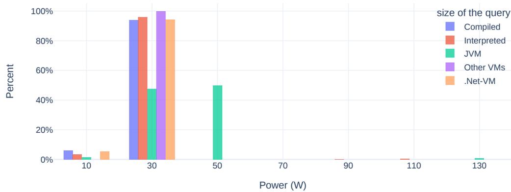
Figure 6.13: Average power consumption for the idle scenario
