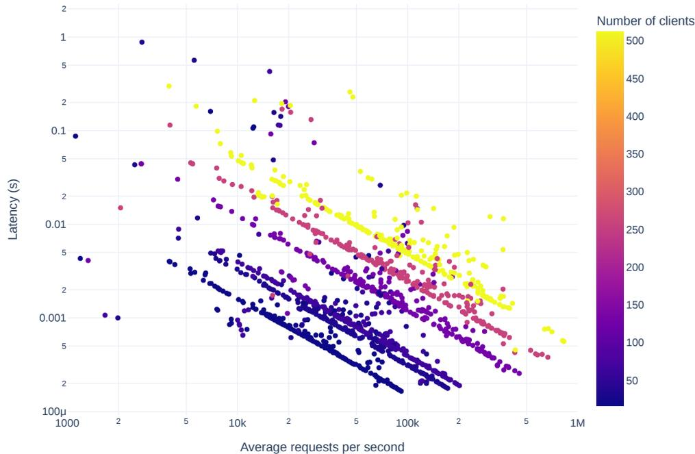
Figure 6.12: Correlation of latency and number of requests per second for a single query
