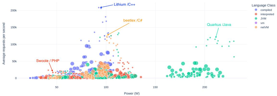
Figure 6.20: Total request vs. average power consumption for the *Update* scenario (size of circles represents the number of clients)
