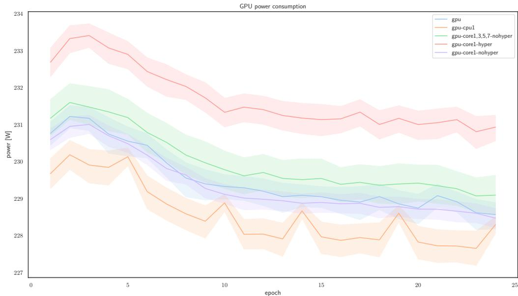
Figure 4.7: Evolution of average GPU power along epochs [73].
