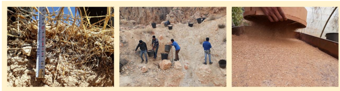
(a) Soil collection at 10 cm depth (b) Soil removal from the site (c) Soil sieving and preparation
