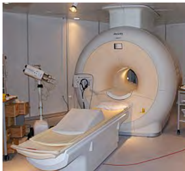
(a) A conventional 1.5T MRI scanner (Philips scanner). Credit: Jan Ainali, (CC BY 3.0), https://commons.wikimedia.org/wiki/File:MRI-Philips.JPG
