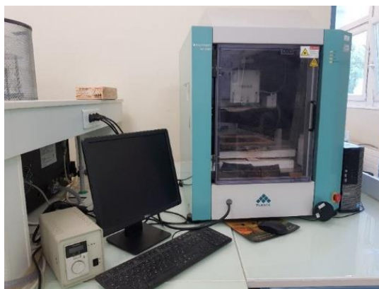
Figure III.1. Electrospinning apparatus Fucec Esprayer ES-2000S2A. All functions are maneuvered by a computer that is connected to the instrument.
