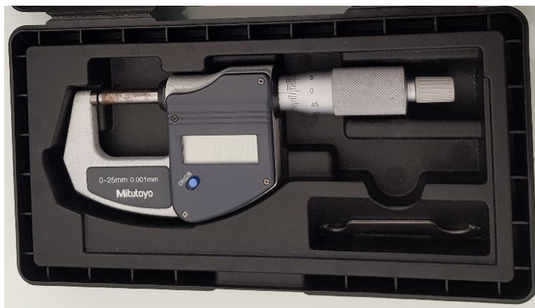
Figure IV.2. Thickness of the compressed textile was manually measured by Mitutoyo Digital Micrometer IP65 Vernier scale.
