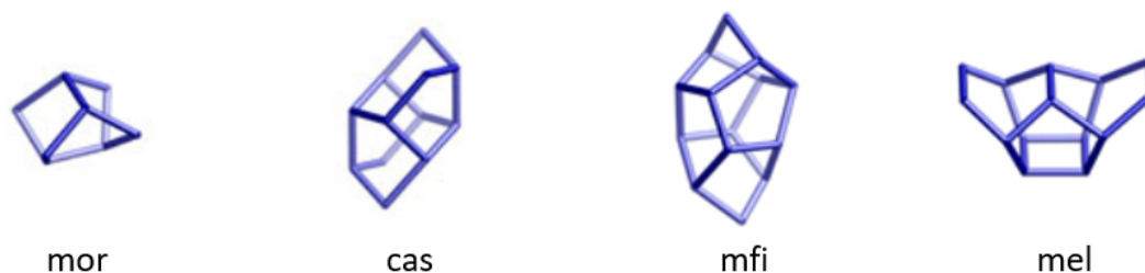
Figure 1.7: Composite Building Units CBU involved in the formation of the MFI zeolite structure. The arrangement of these units allows building channels [42].
