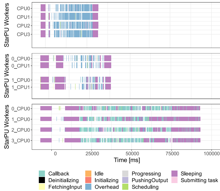
Figure 8.12: Graphical visualization of the execution traces provided by the StarPU runtime corresponding to the execution of HMAT on a FEM system having 25,000 unknowns using (from the top to the bottom of the figure) 1 MPI process times 4 StarPU workers, 2 MPI processes times 2 threads, 4 MPI processes with 1 thread per process on a single miriel node respectively. Blank spaces represent the time spent in computation. The dark violet color indicates sleeping.
