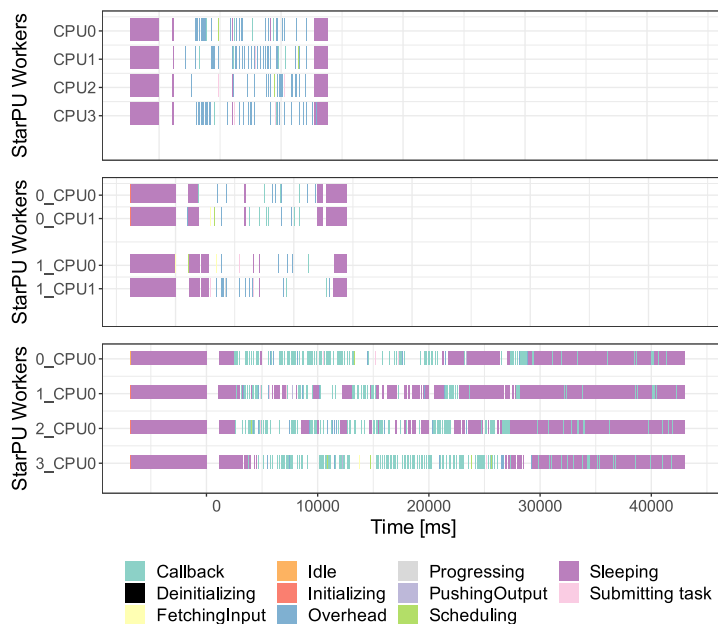
Figure 8.18: Graphical visualization of the execution traces provided by the StarPU runtime corresponding to the execution of HMAT on a BEM system having 25,000 unknowns using (from the top to the bottom of the figure) 1 MPI process times 4 StarPU workers, 2 MPI processes times 2 threads, 4 MPI processes with 1 thread per per process on a single miriel node respectively. Blank spaces represent the time spent in computation. The dark violet color indicates sleeping.
